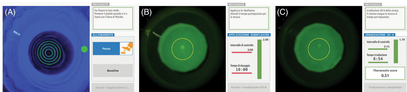
FIGURE 1 Main Thera-CXL treatment steps. A, The device allows the operator to focus onto the cornea to treat with Placido-disc technology; thereafter, the operator acquires the baseline image of the cornea. At preset monitoring time intervals, both during dosing and UV-A photo-therapy phases, the device acquires, processes and calculates the fluorescence emission signal of the cornea illuminated by 3 \text{ mW/cm}^2 UV-A power density for a few seconds in order to estimate the corneal riboflavin concentration. B, The panel shows the measurement of corneal riboflavin concentration at 10 minutes time interval during dosing phase. C, During UV-A photo-therapy, the devices tracks the photo-degradation of corneal riboflavin and calculates the theranostic score providing an estimation of treatment efficacy. The panel shows the measurement of corneal riboflavin concentration and the theranostic score a few seconds before UV-A photo-therapy ending.
